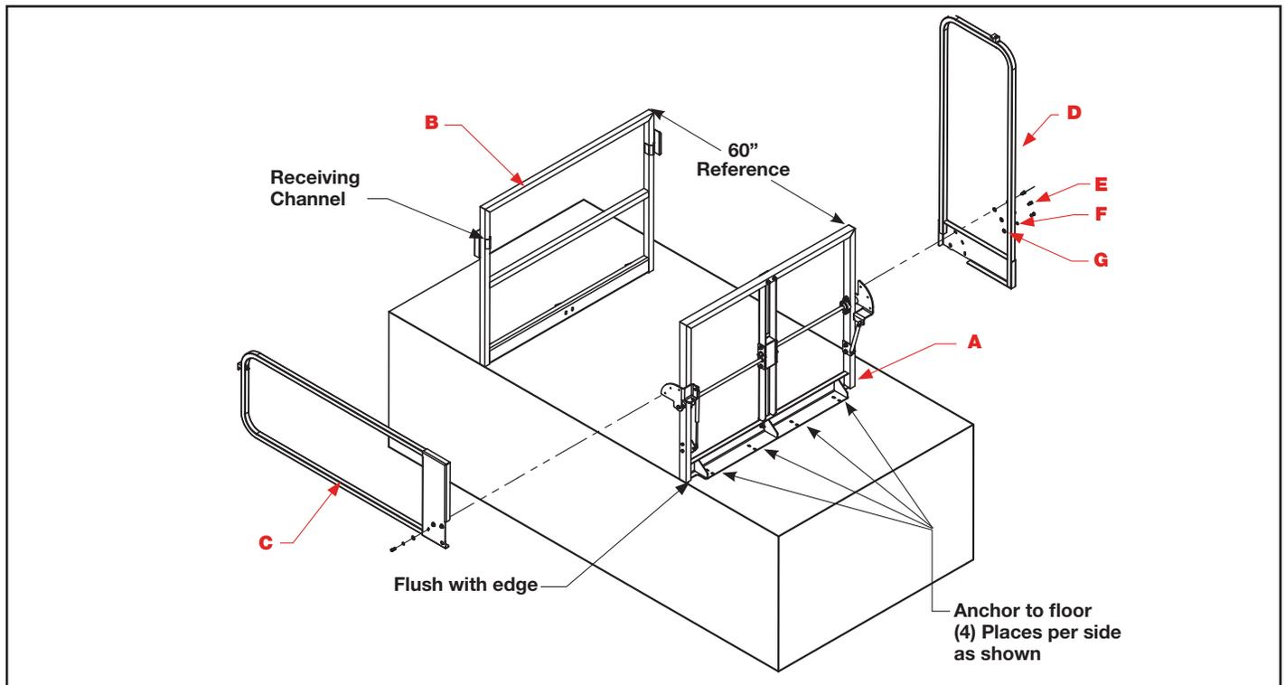
**Safety Note:** There must be OSHA-approved fall protection devices in use during the installation of this product! Assemble the unit away from the edge of the mezzanine. After assembly is complete, move the MZ Clear Height Safety Gate to the edge as shown and anchor to the floor.
