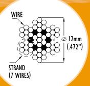
An economical 8mm diameter, 7x7 construction, stainless steel cable with strength exceeding 8,800 lbs. is also available. This system makes it possible to span 30 feet between intermediates and allows up to 2 users. These properties (cable diameter, weight, and strength) are an ideal compromise between safety and aesthetics.
